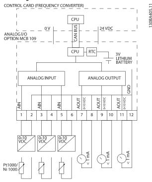
Illustration 5.1 Block Diagram for VLT® Analog I/O Option MCB 109 Mounted in the Frequency Converter.
